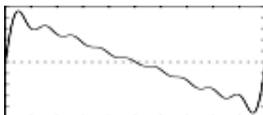
f 1 0 16384 10 1 - sine wave with only the fundamental frequency
